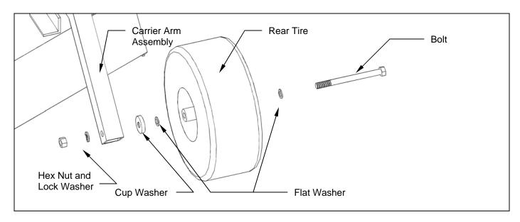
Figure 1: Rear Tire Assembly Installation
